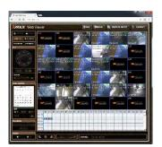
Auto Private IP Setup (NAT Traversal) - Automatically setup a router if you want to connect to the DVR remotely over the internet. The router will need to be setup to support communication to the DVR from an external network by opening the corresponding ports. Settings need to be done individually for each DVR in the network.
