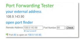
Once the router settings have been configured, open an internet explorer page and enter your router's external IP address:DVR's port number (for example: 72.243.193.215:81).
